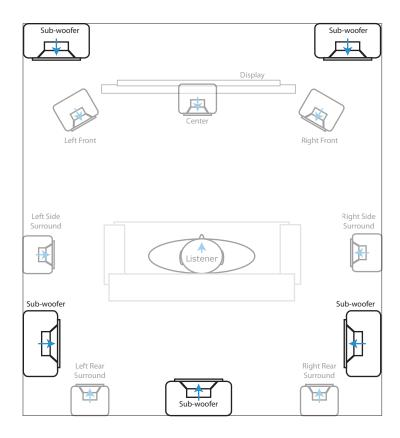
Several factors determine which locations work best for a subwoofer in a given room. The easiest way to get great results is to experiment with different locations until you find the right one. Here are some locations you can try.
